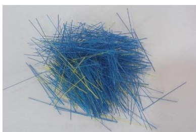
Figure 3. Shape of PP as Plastic Fiber Reinforcement.
